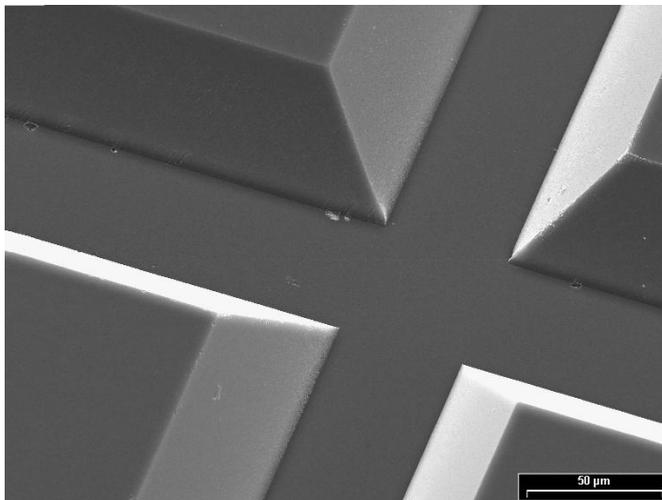
Fig. 4: Channels from electroplated wet etched silicon.
