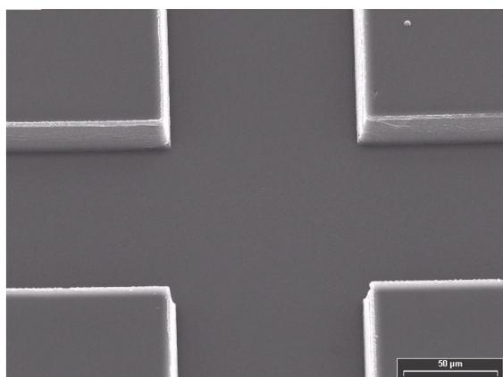
Fig. 5: Channels produced with a Ni-master.
