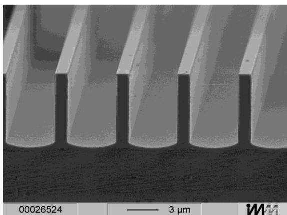
Fig.2: Embossing tool fabricated in silicon with ASE.
