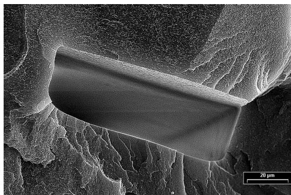
Fig. 6: Cross-section of a channel with a bonded cover lid. Note the absence of a visible interface between channel plate and cover plate.
