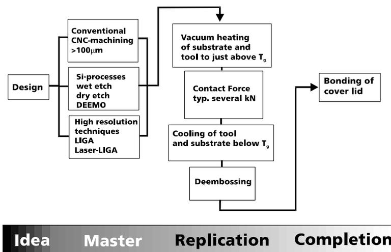
Fig. 1. Schematics of the fabrication process.
