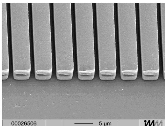
Fig.3: Resulting channel structure.
